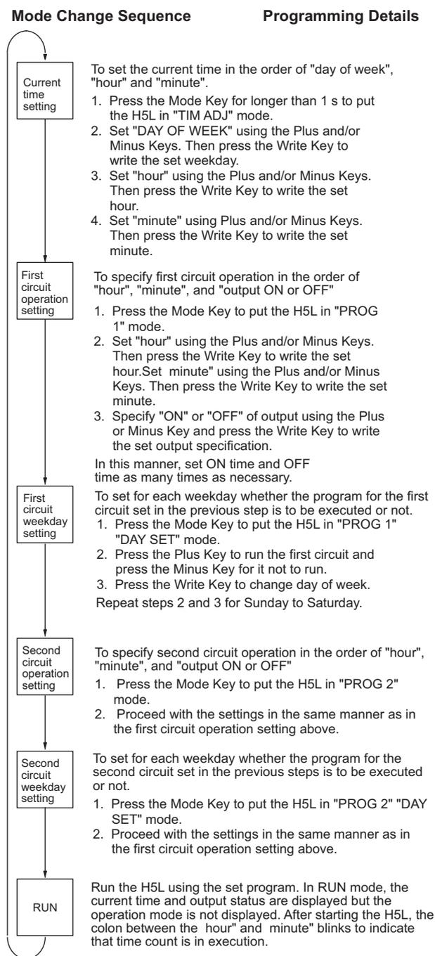
**Note:** The H5L operates in accordance with the program already set even while another program is being set. The output status display (ON/OFF etc.) during programming displays the setting being programmed. Therefore, note that the output status displayed on the LCD may not agree with the actual output status.
