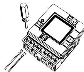
**Note:** Screw tightening torque: 0.98 N·m max.
